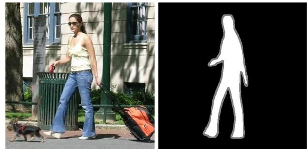
Fig. 4. Sample trimap of a pedestrian. White pixels represent confirmed object, gray pixels represent mixture of object and background and black pixels represent confirmed background
