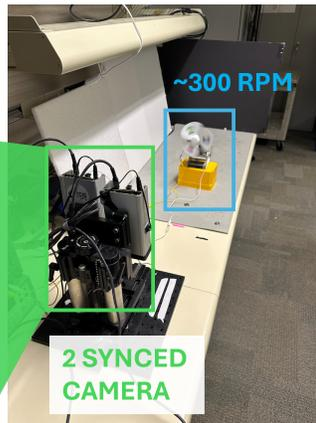
Fig. 3. Hardware setup for passive stereo imaging, designed to capture hybrid scenes featuring both static and dynamic objects.
