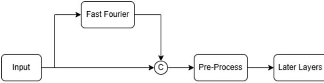
Fig. 4: Fourier Channel's Pipeline
