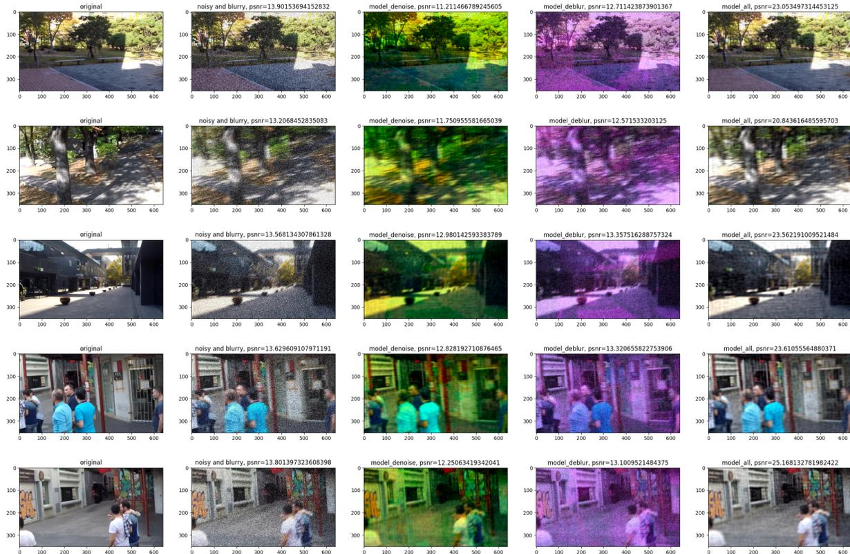
Fig. 6. Comparison between FA-UNet, Denoise Net and Deblur Net. From left to right, each column includes the original high-quality images, noisy and blurry images, images after being processed by the Denoise Net, images after being processed by the Denoise Net, and images after being processed by FA-UNet.
