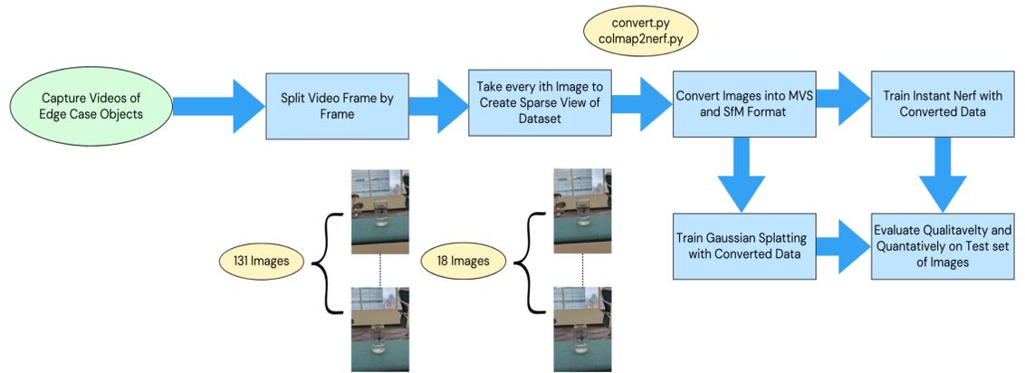
Figure 3: Reconstruction Workflow
