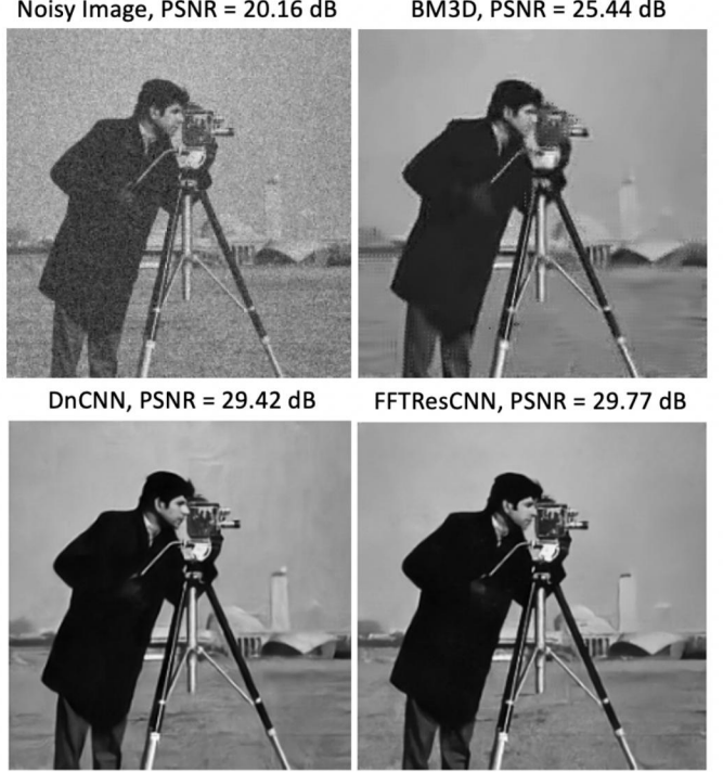
Fig. 10: BM3D vs. DnCNN vs. FFTResCNN: final denoising results of one image from the test dataset ( \sigma = 25 )
